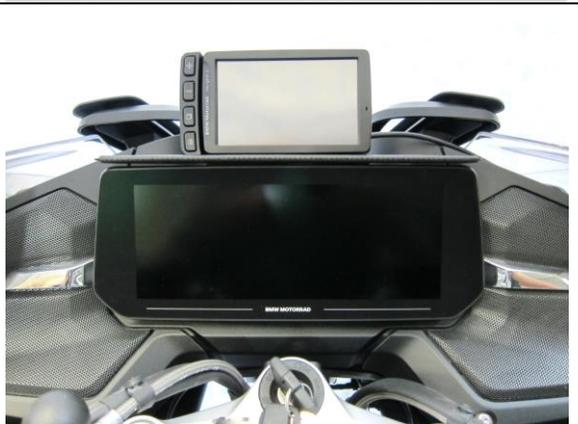
If you are connecting a GPS cradle / mount that is not from BMW, you likely do not have the 3x connector needed to plug into the GPS plug located behind the motorcycle dashboard. Remove fairing speaker to access plug.
