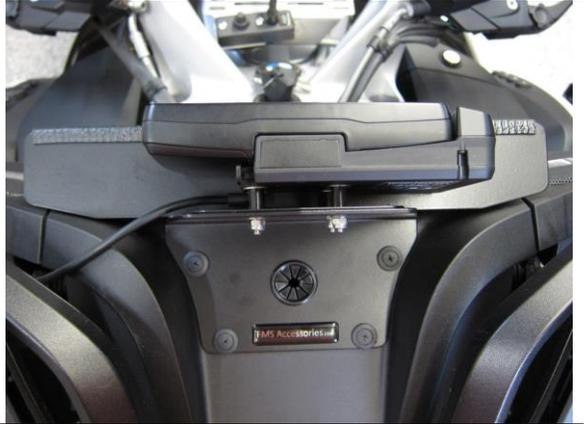
It is recommended to route your GPS power cable down through the center hole designed for cable entry. If routing outside, be careful to not block the isolation damping of the TFT screen, etc.
