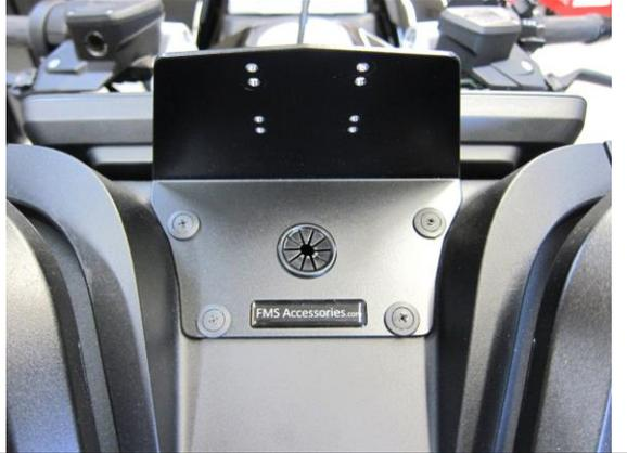
The FMS BMW NAV cradle mount has two sets of indexed holes to enable use of either the BMW four-button cradle or the later locking cradle from the GS / ADV series motorcycles.
