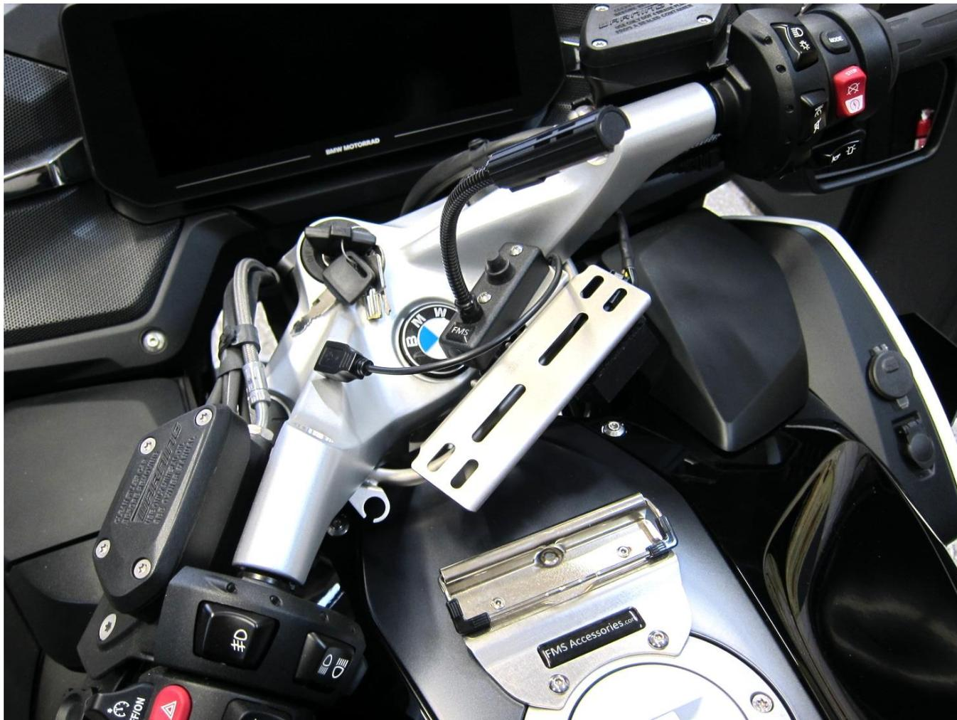
The FMS Cell Phone Power Converter is designed to provide power to your cell phone or charger base utilizing the map light power plug under the RH handlebar, rather than connecting to the USB / Voltmeter socket in the fairing.
