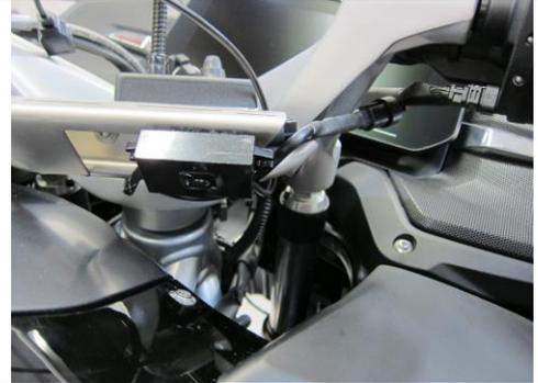
The map light plug has a release tab. Press down on the end of the tab to release the pin housing from the plug. On new motors, there is a waterproof cap on the hanging plug. Press down and release the cap to enable connection of the phone charger.
