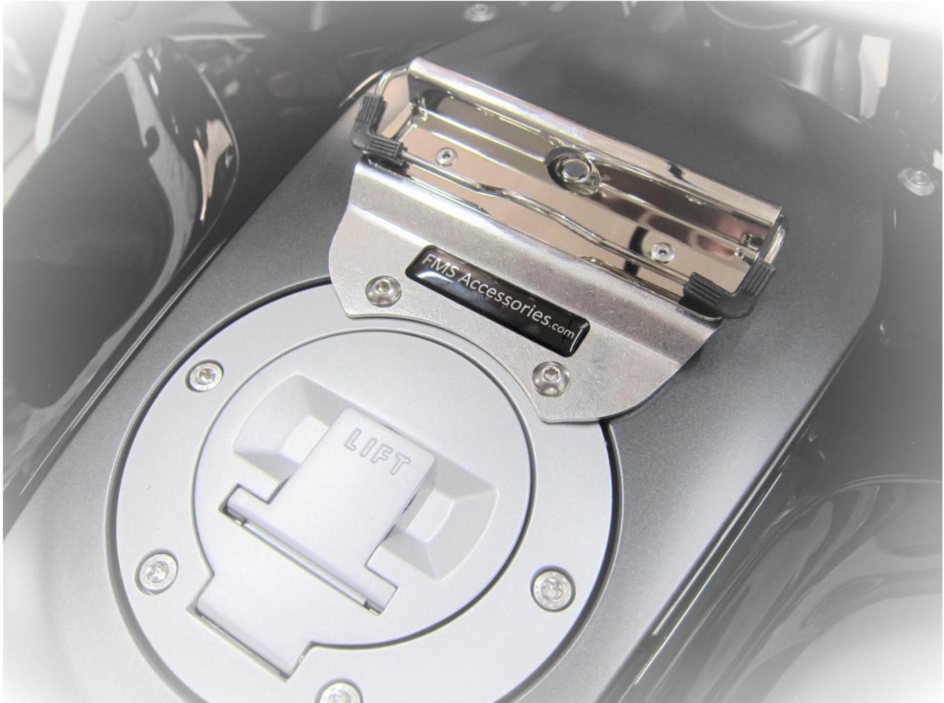
Remove the two M5 x 28 mm T25 Torx bolts securing the front of the fuel filler cap ring.
