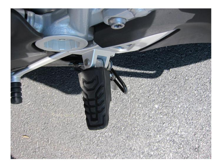
Extend the side stand and slide the tapered extension over the stock side stand foot. Tap lighting to ensure it is seated. Using a ¼" drill bid, drill through the side stand foot using the extension as a guide.
