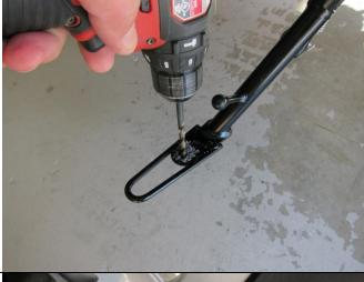
Deburr the hole from the bottom-side of the stand.
