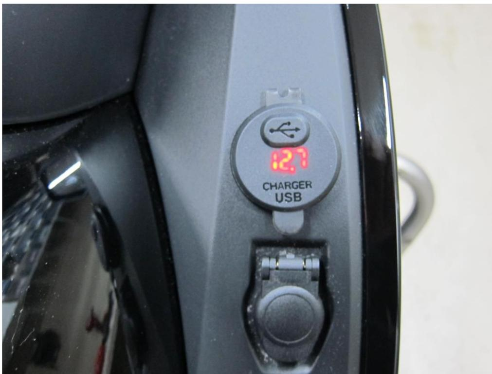
FMS Accessory USB / Voltmeter can be connected in three different methods.
