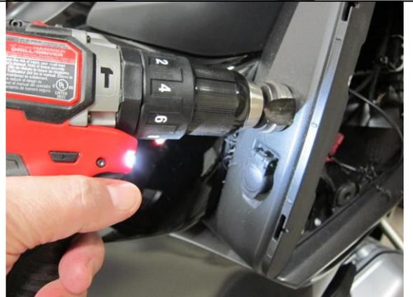
Install USB through hole, install nut behind and tighten, correcting plug and weatherproof cover alignment as desired.
