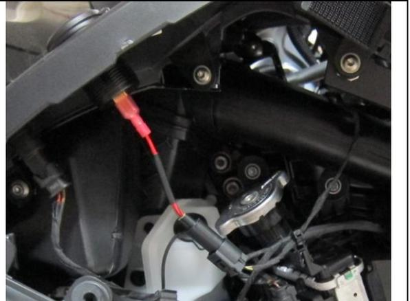
Insert the harness plug into the speaker outlet (6X) and then select ACC II or ACC III for the other end of the harness.
