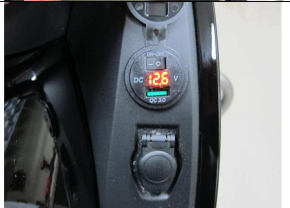
For connection to the accessory power socket, connect the supplied harness to the USB (red = + / brown = -). Remove the Hirschmann connector from the existing accessory power socket and connect that lead to the mating plug on the "Y" harness at right. Connect the other mating "Y" harness plug to the accessory power socket. With this connection, the socket should shut-off 50 seconds after ignition-OFF.
