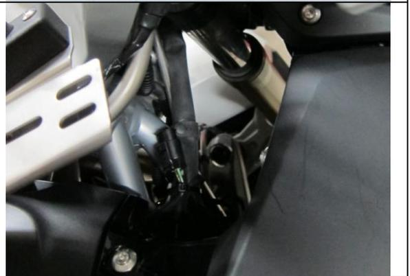
Route the cable past the air intake tube and plug into the pigtail harness from the USB outlet. Secure the harness by replacing the cable tie on the radiator with the one provided capturing all three cables at that point.
