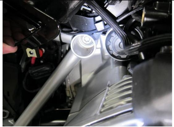
Route the cable up behind and intake tube and coolant expansion tank. Secure onto existing wiring harness.
