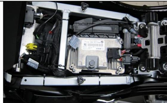
Pull black trim panel away from fuel tank edge and run cable along frame support, through the plastic guide, behind the braided fuel line and behind the throttle body.
