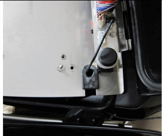
Remove seat bolster by loosening the two thumb nuts, then pulling the bolster forward. As the radio box unlock switch cable will still be connected, it is best to open the LH saddlebag and place the seat bolster in there so that the cable is not damaged.
